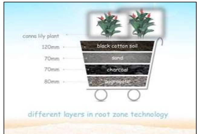
Fig. 1.5: Different Layers in Root Zone Technology (A. A. Raval and P. B. Desai, 2015)
