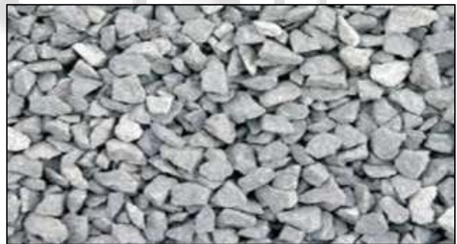
Fig. 3.5: Aggregate i.e. gravel layer to be provided because the bottom-most layer of the basis zone treatment system for straightforward filtration of the waste effluent.
