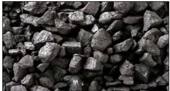
Fig. 3.4: Coal makes the foremost important layer in root zone treatment system acting because the waste absorbing agent, layer to be provided below sand layer.
